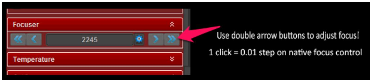
Focus control can be seen in the Firecapture sidebar. Use the **DOUBLE ARROWS** to make focus adjustments as this corresponds to the smallest step on the native focus control.
