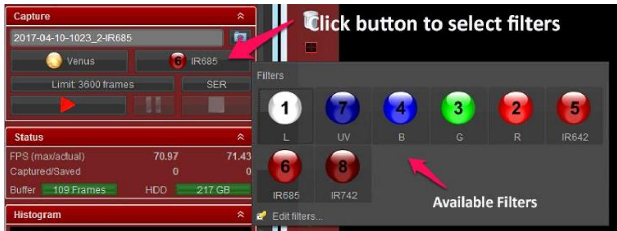
To select filters simply click the filter button indicated to bring up the selection available. Again note Firecapture will automatically refocus for each filter one you have calibrated the focus positions.
